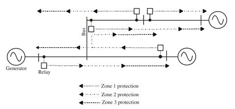
Figure 2-9: Protection zones of a transmission line
