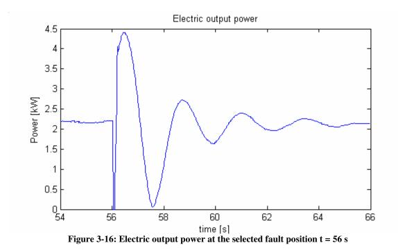
The duration of the fault drawn in Figure 3-16 was 500 ms.
