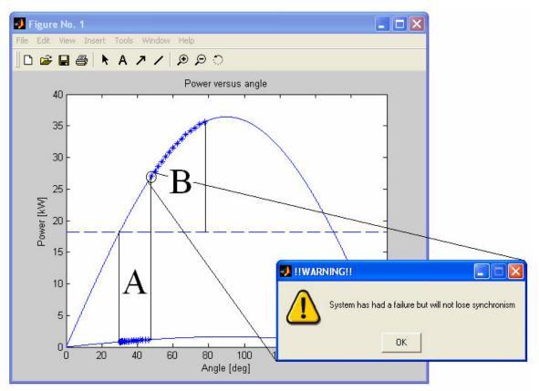
Figure 3-20: Fault is cleared before the critical fault clearing time
