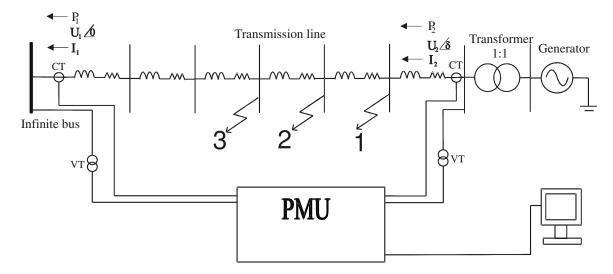
Figure 3-14: Lab setup with fault at three different locations
