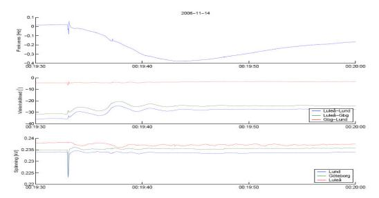
Figure 2-7: Voltage, voltage phase difference and frequency recordings 14th of November 2006
