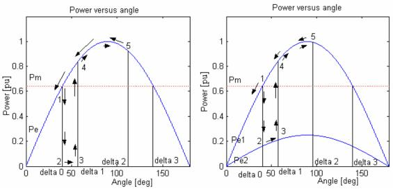
Figure 2-4: Power transfer before, during and after a fault close to the turbine-generator Left diagram: Electric power output decrease to zero during fault. Right diagram: Electric power output decrease to  $P_{e2}$  during fault.
