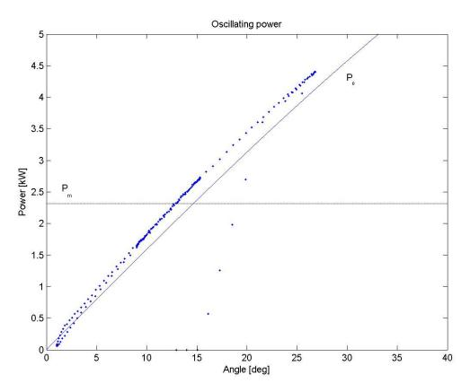
Figure 3-19: Power oscillation when recovering from fault
