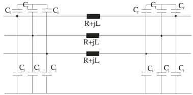
Figure 3-2: Resistance, inductance and capacitance of one  $\pi$ -section
