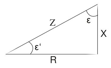
Figure A-2: Impedance angle and loss angel
