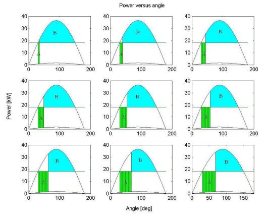
Figure 3-12: Riemann integration for equal-area criterion
