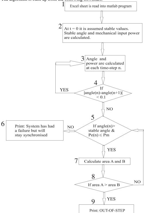
The algorithm is built up from the following flowchart:
