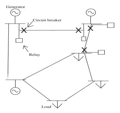
Figure 2-6: Meshed power system
