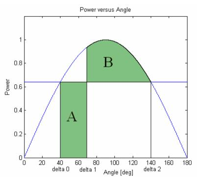
Figure 2-5: Equal-area criterion with an acceleration area A and a decelerating area B
