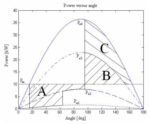
Figure 3-23: Electric power output, before fault, during fault and after fault is cleared
