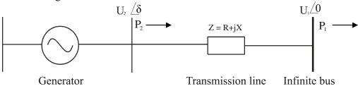
Figure 2-2: One machine against infinite bus diagram
