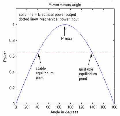
Figure 2-3: Input (dashed) and output (solid) power of a turbine-generator
