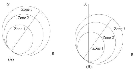
Figure 2-8: Mho and offset mho characteristics
